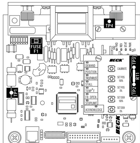
Location of DCM-2 Test Points and Resistor 11
