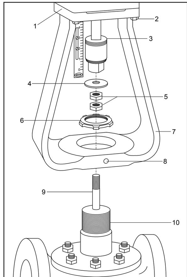
5. Place the jam nuts (5) and travel index (4) over the valve stem (9) before mounting the drive on the valve.
