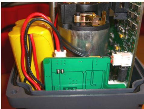
The main advantage of **J+J's** BSR system is that it is more competitively priced compared to mechanical spring return actuators, as the **J+J** actuator has no mechanical springs to compress, or solenoids to release them - the actuator is the same size as that for an on-off version. This offers massive savings compared to true mechanical spring return electric actuators.
