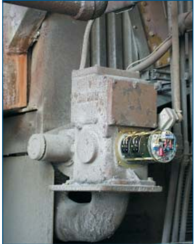
Individual compartments protect components
