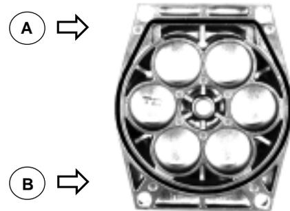
**6.9 -** In case of SPRING RETURN actuator insert cartridge springs. (For information on the loading of springs refer to section 7.0).
