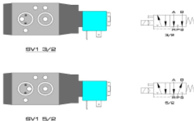
In addition to these 4 standard models of solenoid valves, with nylon fiberglass filled coils, G.T. Attuatori offers also Epoxy Resin filled coils, for all standard voltages and also for other voltages, when request, always with same consumption data.
