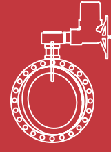
L120/WTR mounted to butterfly valve
