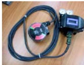
Acrodyne has taken the next step in transferring the sensor device to an IP67 housing thus giving ideal protection in corrosive areas. The housing includes a stainless steel namur shaft which can be easily adapted to linear operation.
