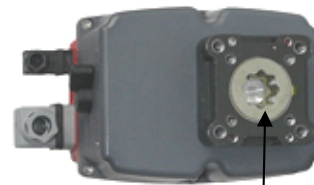
Models: J3-55 and J3-85 Mounting: F05, and F07 50mm and 70mm PCD Output: 17mm double square (star) 14mm option
