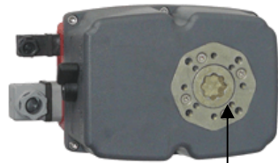
Models: J3-20 and J3-35 Mounting: F03, F04 and F05 36mm, 42mm and 50mm PCD Output: 14mm double square (star) 9 and 11mm options
